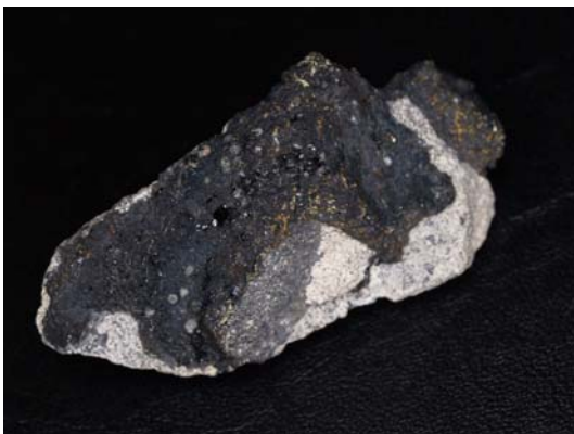
Redbank transitional copper ore specimen (view 2 cm across).
